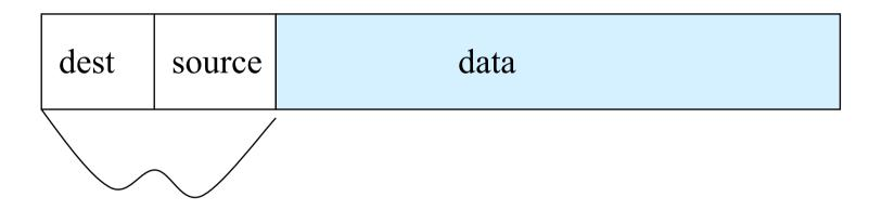
Ethernet header: 6 byte addresses – strangely large...because it allows autoconfiguration Plus stuff like protocol type and VLAN
