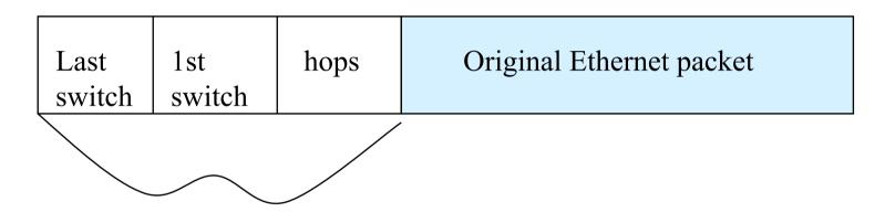
TRILL header Switch addresses are 16 bits
