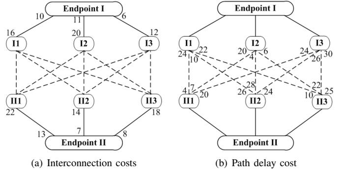
Fig. 2. Multihoming example with 18 subflows
